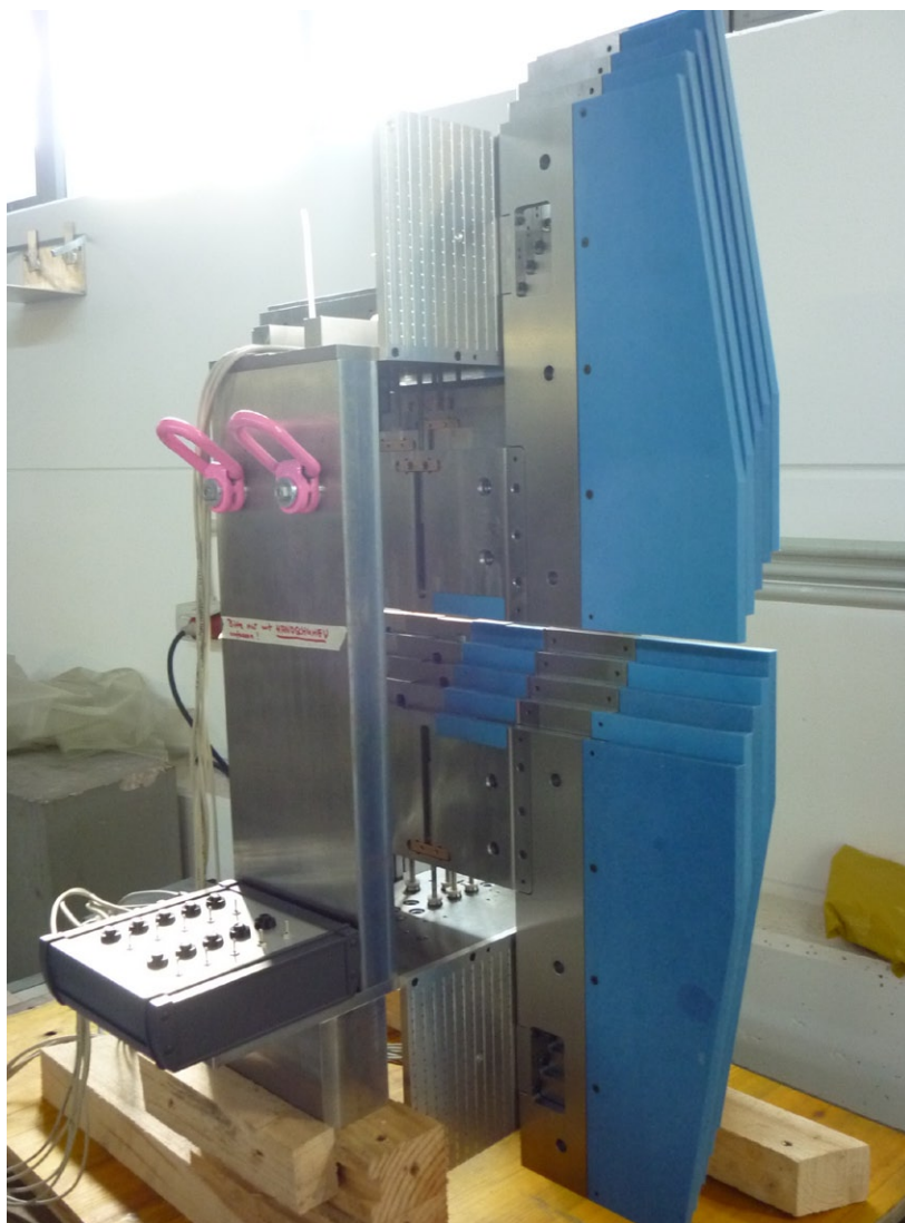
Fig 6. Prototype of a new collimator for MEDAPP.
